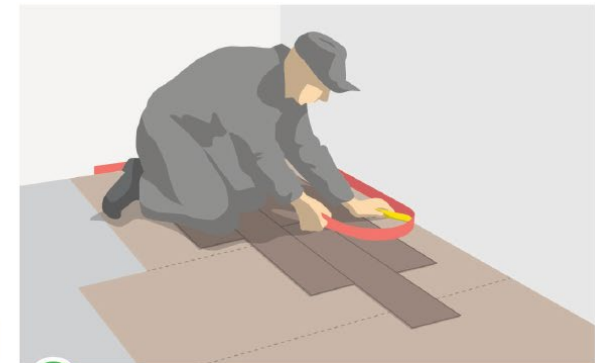
6 Perimeter insulation barrier cut
