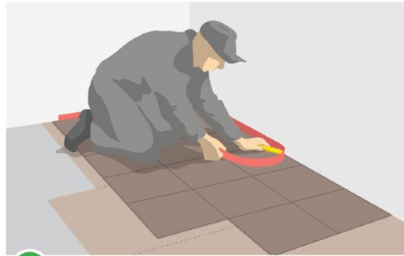
4 Perimeter insulation barrier cut
